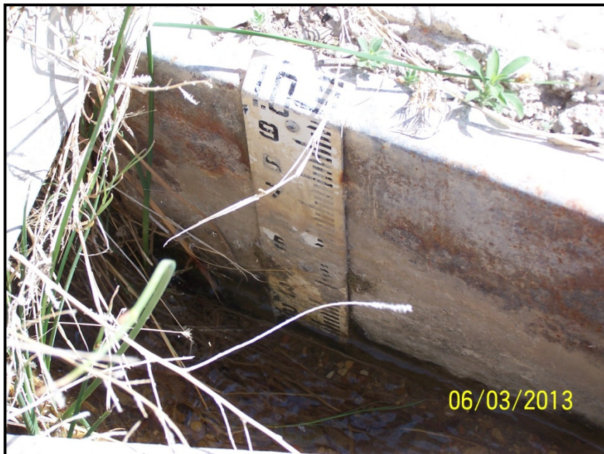
Photo 8 — USGS gauging station between Wetlands WCN-1 and WCS-1 on Williams Creek.
